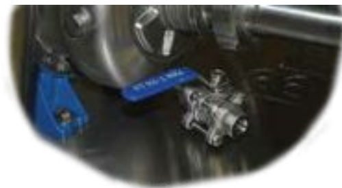
Function 10: Lowest point cleaning system.
